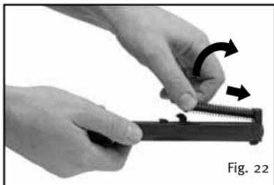
10. Press the recoil spring toward the front of the slide while pulling it up to remove it from the slide.
