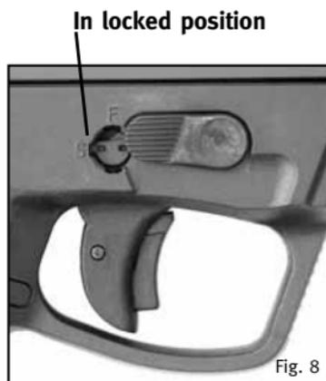
The integrated limited access lock is manually operated by using a separate key. When locked, it locks the trigger and prevents the disassembly of the pistol. The integrated limited access lock can only be locked when the pistol is cocked (trigger in the forward position).
