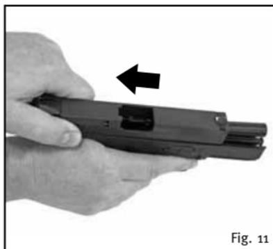
2. Retract the slide to eject any cartridge that may be in the chamber.
