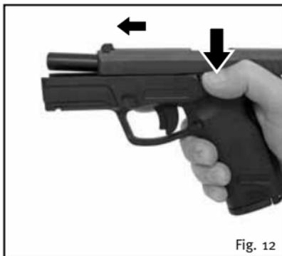
5. Release the slide to return it to the forward (closed) position.
