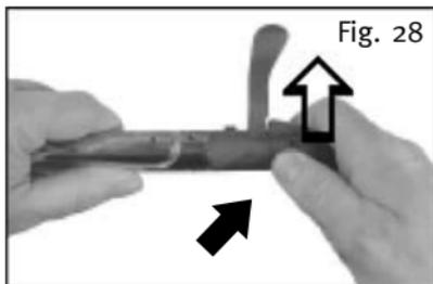
1. Grip the bolt with your left hand. Push in catch lever with your right thumb and simultaneously rotate the bolt sleeve clockwise (arrow shows direction of rotation) until it unlocks with an audible click.
