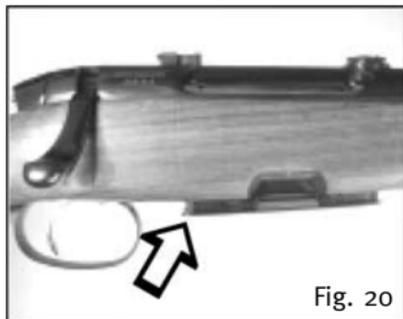
2. Remove magazine or lock it in second position (magazine protrudes by approx. 5 mm/ 0,19").
