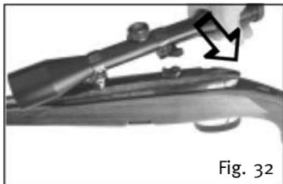
Hold the scope with your right hand in horizontal position, at an angle of  $45^{\circ}$  to the rifle axis, mount the front scope ring (for prism mounts this part is termed holding prism) on the front base and swing the scope in a clockwise direction until it locks automatically. Pulling back the slide is not necessary.
