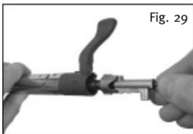
2. Take off bolt sleeve and extract firing pin assembly.
