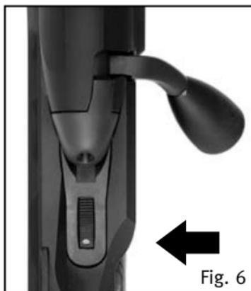
Release safety only shortly before firing the shot. If the weapon has to be reloaded after firing a shot, the bolt handle must be opened.
